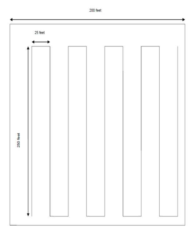
Figure 1: Landfill Walk Pattern for an Ideal 50,000 Square Foot Grid
